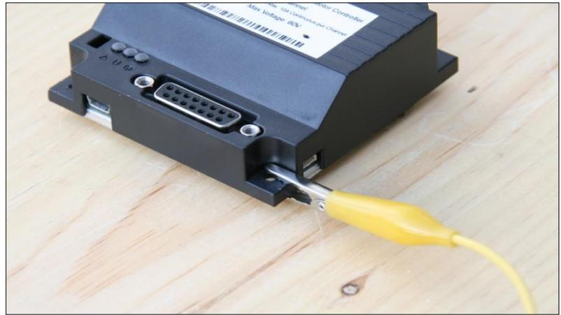
Bleeder resistor connecting conduction plate to reference plane
