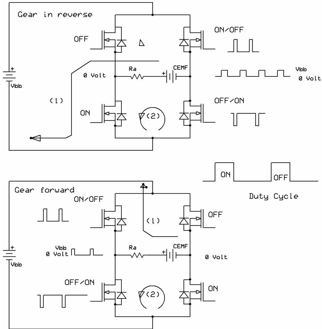
(1) Current loop during duty cycle ON time
