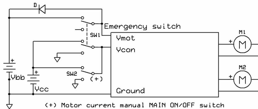
(B) LARGE MOTOR CIRCUIT WITH CONTACTOR EMERGENCY SWITCH
