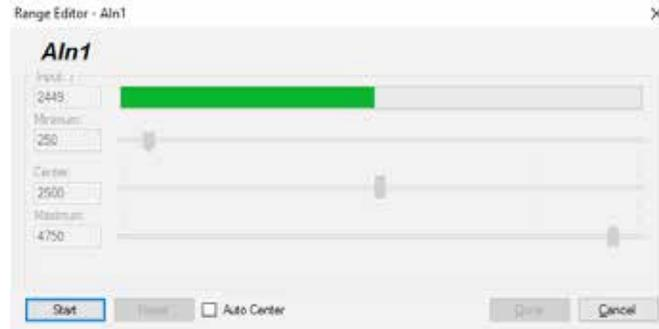
After clicking on the “Done” button, the capture values will appear in the Min, Max and Center nodes in the tree with the orange \* next to them, indicating that they have changed but not yet be saved in the controller. At this point, they can be adjusted further manually and saved in the controller.
