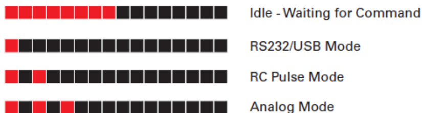
FIGURE 8. Normal Operation Flashing Patterns
