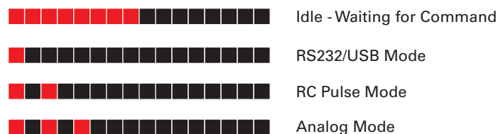
FIGURE 13. Normal Operation Flashing Patterns
