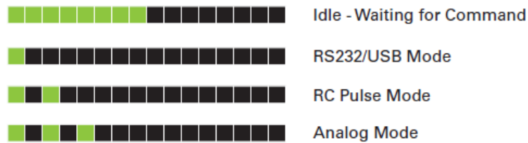
FIGURE 8. Normal Operation Flashing Patterns
