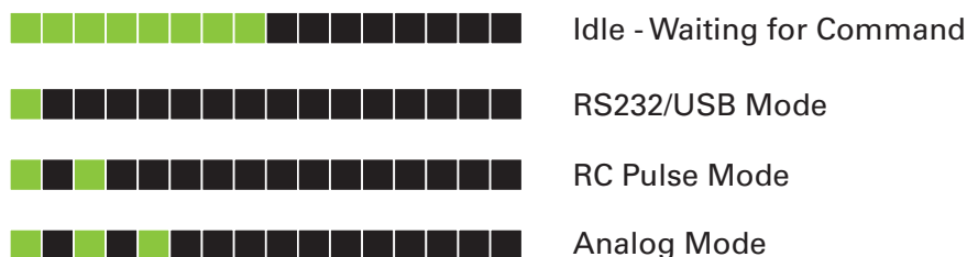
FIGURE 9. Normal Operation Flashing Patterns
