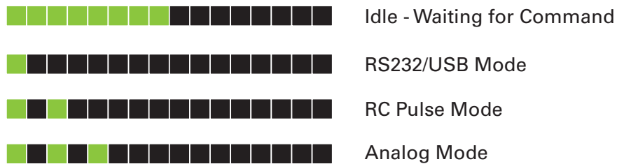
FIGURE 9. Normal Operation Flashing Patterns
