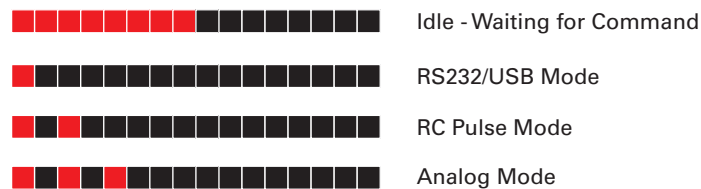
FIGURE 9. Normal Operation Flashing Patterns
