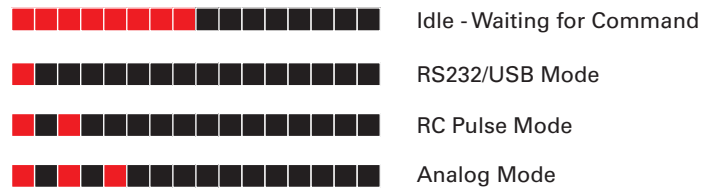
FIGURE 9. Normal Operation Flashing Patterns
