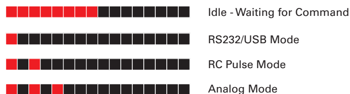
FIGURE 15. Normal Operation Flashing Patterns
